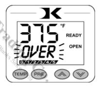
If the OverTemp alarm sounds, set the temperature to a higher value than the current actual temp. Wait 30 seconds and then reset the press to your desired temperature and Watch Carefully. Do not let the press rise to extremely high temps.
